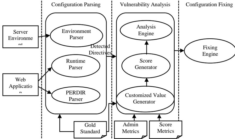
Figure 3: Workflow of the proposed tool
