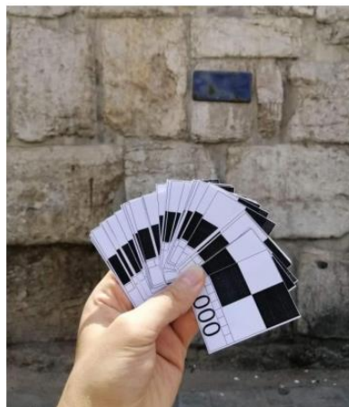
Figure 29: Control Points (markers) example
