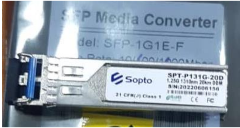
الشكل (3-3) - small form-factor pluggable (SFP)
