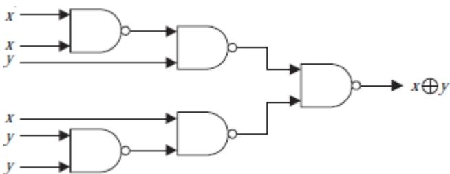
$$\overline{\overline{\overline{xy} \overline{xy}}} = \overline{\overline{(x+y)(\overline{x+y})}} = \overline{\overline{(x+y) + (\overline{x+y})}} = \overline{xy} + \overline{x\overline{y}}$$
