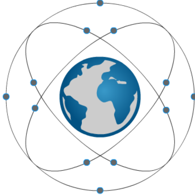
(b) Medium earth orbit: inclined to the equator, at 5000 to 18,000 km altitude
