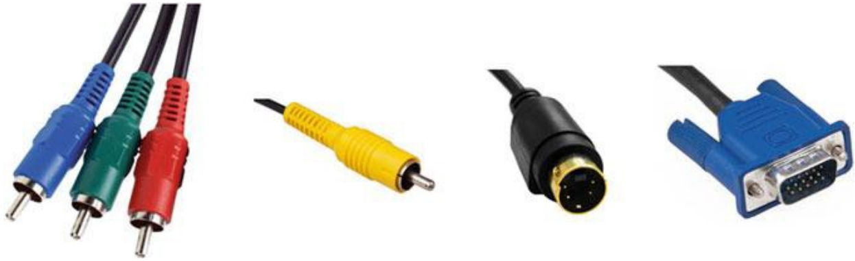
Fig 6–3 Connectors for typical analog display interfaces. From left to right: Component video, Composite video, S–video, and VGA
