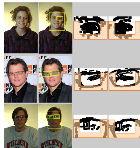
Fig. 14. Statistical glasses detection method implementation examples, skin color result (blue rectangle), Viola-Jones result (yellow rectangles) glasses detection (green rectangle)
